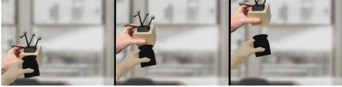
FIGURE 3 Illustration of applying pseudo-haptics for weight perception in VR. The manipulation of the offset between the rendered hand position and the actual hand movement lead to an impression of different weights [64].
