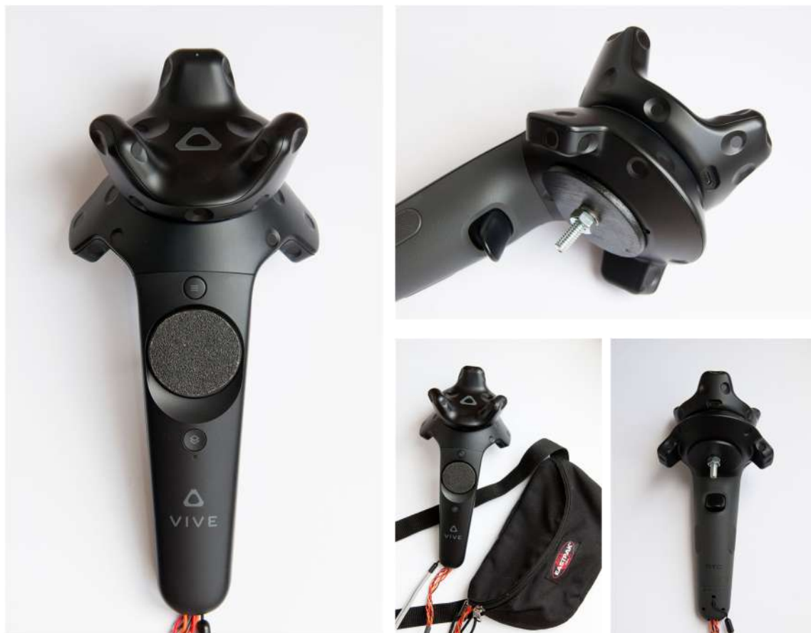
FIGURE 16 The final version of the first prototype with an attached Vive tracker for spatial tracking. The cables are connected to the electrical components inside the bag.
