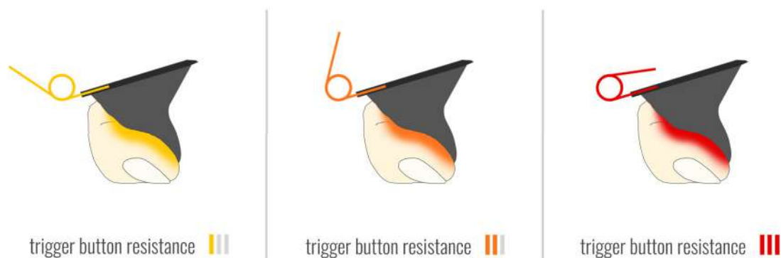
FIGURE 7 A torsion spring with three different angles exerting three different levels of torque. The respective trigger button resistance is a direct result of the torsion spring's modification.
