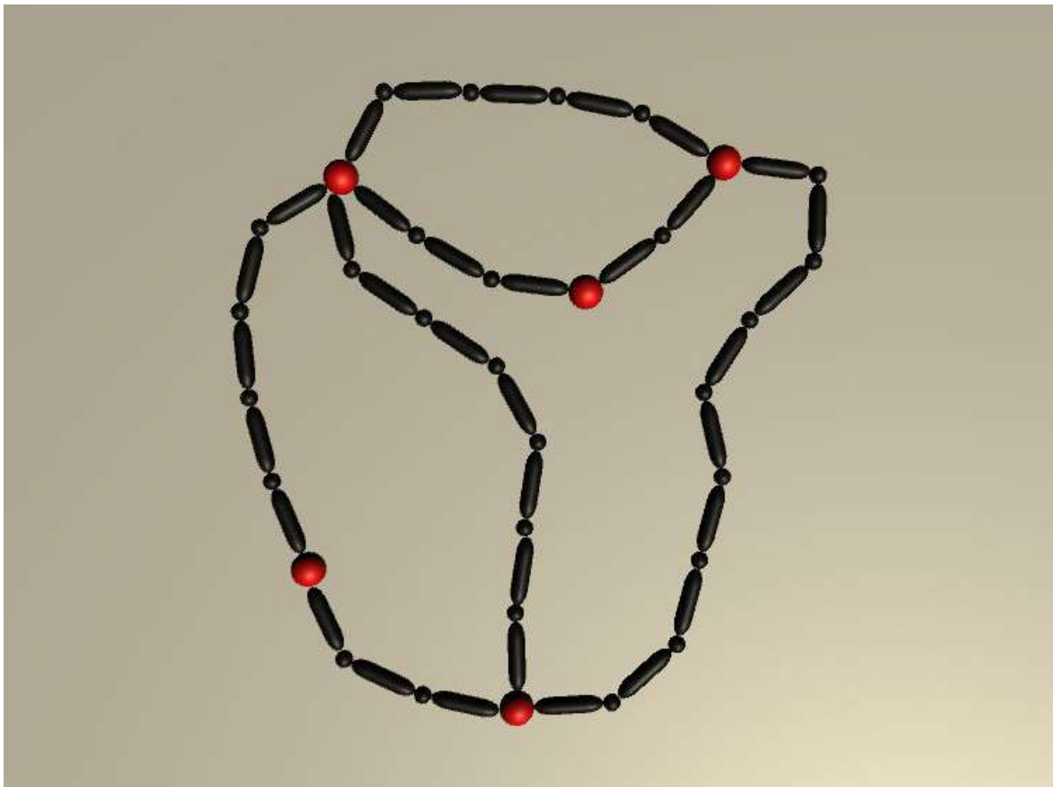
Figure 5: Simulated rope forming a net. Components of the rope are waypoints (red), as well as capsules and spheres (black). The simulation is shown in its resting state.
